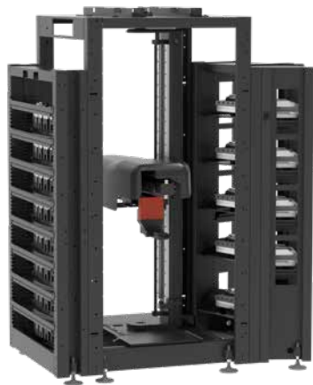
Two magazines example • One light magazine 8 levels with 10 pallets/level • One Heavy magazine 5 levels with 2 pallets/level Summary 80 Macro 54 pallets 10 Dynafix 350 pallets
