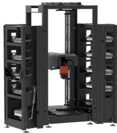
Two magazines example • Two heavy magazines 10 levels with 2 pallets/level Summary 20 Dynafix 350 pallets
