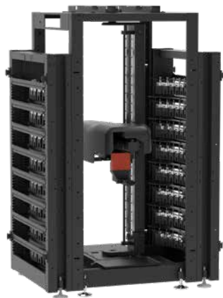
Two magazines example • Two light magazines 16 levels with 10 pallets/level Summary 160 Macro 54 pallets
