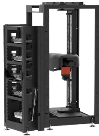
One magazine example • One heavy magazine 5 levels with 2 pallets/level Summary 10 Dynafix 350 pallets
