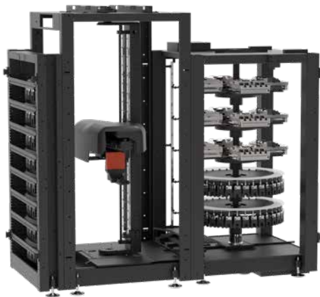
Two magazines example • One light magazine 8 levels with 10 pallets/level • One rotary magazine 2 levels with 36 pallets/level 3 levels with 4 pallets/level Summary 152 Macro 54 pallets 12 Dynafix 350 pallets
