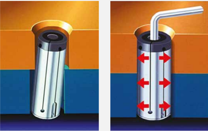
3Refix expanding mandrels (2 pcs) determines the position. First 3Refix mandrel is to determine X/Y-position and the second to determine the angle.
