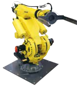
Automation – with 6-axis industrial robot
