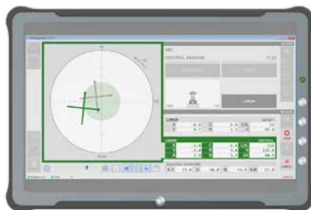
Check tilt of chuck as a verification.
