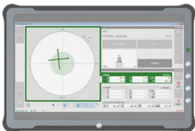
Adjust location of chuck until displayed area turns green.
