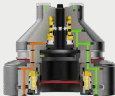
Chuck adapter connectors – unclamping and Turbo/air-blast cleaning
